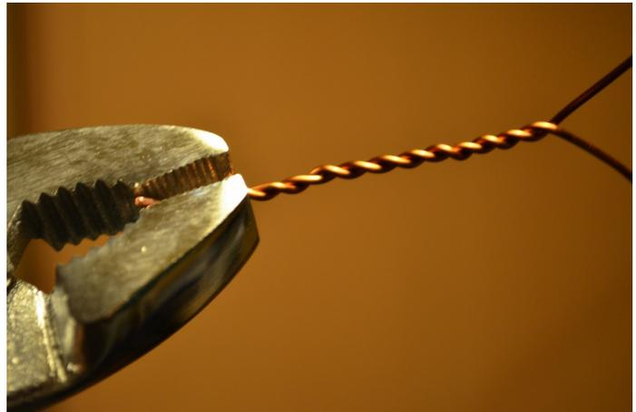
If using an FT240-43, start by measuring out two pieces of 20SWG enamelled copper wire – one is about 1m, long and the other about 22cm. Twist the two together for the first 130mm, ensuring that you do this neatly. The twisted section then makes up the two bifilar turns on the primary.
