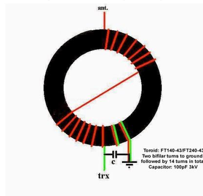
somewhere between 2000-5000 Ohms. In some designs, my earlier ones included, we make a resonant circuit using a toroid coil and capacitor to resonate at the frequency required.
